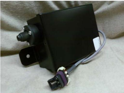
An optional TCI® SCU uses an electric motor to spin a special speedometer cable to drive a mechanical speedometer. The SCU wiring mates directly to the EZ-TCU™ wiring harness.
